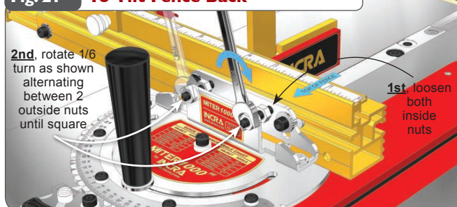
Fig. 21 To Tilt Fence Back
