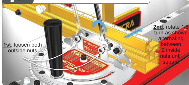
Fig. 20 To Tilt Fence Forward
