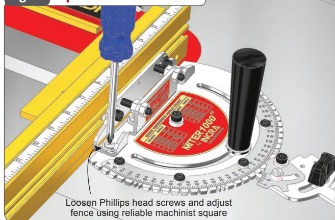
Fig. 8 Square Fence to Blade
